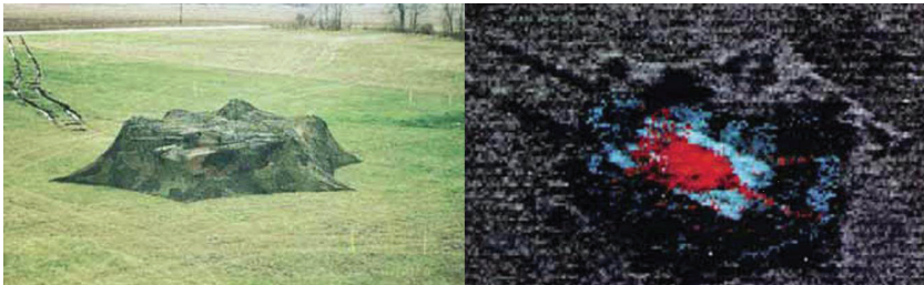
FIGURE 11.6 Laser Radar Image of a Tank under Camouflage Netting
