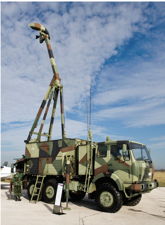
FIGURE 3-13 Giraffe Battlefield Surveillance Radar
