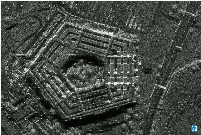
FIGURE 7-1 Airborne SAR Image of the Pentagon
